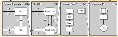
BLOCK keyword. The blocks diagram contains a number of Processes and may also possibly contain other BLOCKs (but not mixed with Processes). Processes communicate via Signal Routes, which connect to other Processes or to Channels external to the Bloc
